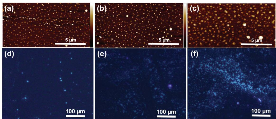
**Fig. 3** AFM height images (a–c) and fluorescence microscopy images (d–f) of PAN brushes grafted from silicon substrates by photoinduced ATRP using 50 ppm (a, d), 200 ppm (b, e) and 400 ppm (c, f) of copper catalyst; z-scales are 20 nm, 15 nm and 35 nm in (a), (b), and (c), respectively.
