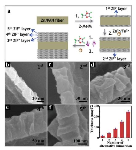
Fig. 3 (a) Cross-sectional illustration of LBL growth of ZIF' layers on Zn/PAN fibers. (b-f) FESEM images of ZIF' shells obtained with different numbers of alternate immersion. (q) Correlation between the average thickness of ZIF' shell and the number of alternate immersion.
