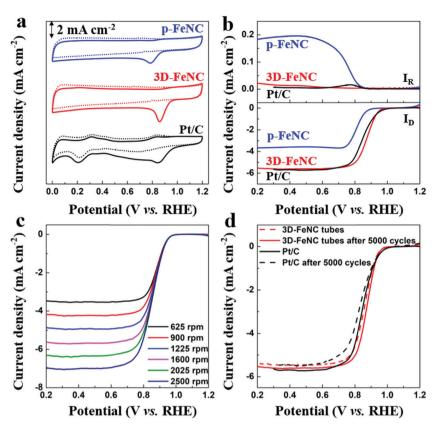
Fig. 5 (a) CV and (b) LSV curves of p-FeNC, 3D-FeNC, and Pt/C catalysts at 1600 rpm in  $N_2$  (dot line)/ $O_2$  (solid line)-saturated 0.1 M KOH solution. (c) LSV curves of the 3D-FeNC catalyst in  $O_2$ -saturated 0.1 M KOH solution at different rotating speeds. (d) LSV curves of the 3D-FeNC and Pt/C catalysts before and after 5000 cycles in  $O_2$ -saturated 0.1 M KOH solution at 1600 rpm. The scan rate is 10 mV s<sup>-1</sup> for LSV curves in (b-d).
