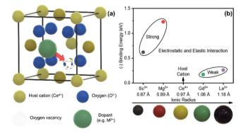
Fig. 1 (a) Schamatic illustration of a unit cell of fluorite structured ceria, showing electrosteric interaction between the acceptor dopant and charge compensating oxygen vacancy. (b) Computationally calculated binding energy (1nn) values of variously doped ceria as a function of dopant radius. The data are taken from V. Butler et al.<sup>24</sup>
