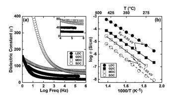
Fig. 2 (a) Estimation of dielectric constant with respect to frequency, measured via EIS at room temperature under AC bias of 10 V. (b) The temperature-dependent Arrhenius plot for the total electrical conductivity of variously doped ceria samples, examined in air.
