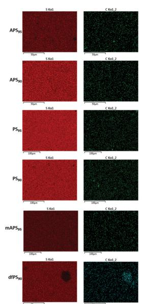
Fig. 2 Surface analysis of biomass—sulfur composites by EDX revealed the homogeneous distribution of sulfur (left) and carbon (right) for biomass—sulfur composites. Voids in the sulfur map where high carbon content is observed are identified as unreacted peanut shell particles in the physical blend dfPS<sub>90</sub>.
