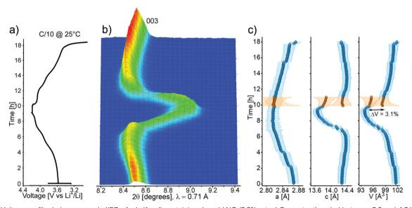
Fig. 6 (a) Voltage profile during operando XRD of a half-cell containing doped LNO (2.2% actual Ga content) cycled between 3.0 and 4.3 V vs. Li<sup>+</sup>/Li. (b) Contour plot showing the evolution of the 003 reflection. (c) Corresponding variation of the lattice parameters a and c and the unit cell volume V. Blue squares and orange circles denote monophasic and biphasic regions, respectively
