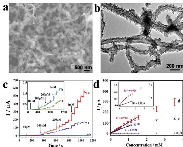
Fig. 5 (a) SEM image of NiCoO<sub>2</sub>@CNT. (b) TEM image of NiCoO<sub>2</sub>@CNT. (c) Amperometric responses to the successive additions of glucose. (d) The calibration curves obtained in the 0.1 M NaOH/NaAc buffer (pH 12.0). Reproduced ref. 47 with permission from Elsevier B.V., copyright 2015.
