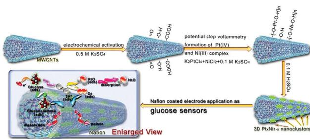
Fig. 12 Schematic diagram of the synthesis and reaction mechanism of the glucose sensor based on the flower-like 3D Pt<sub>x</sub>Ni<sub>1-x</sub>/MWCNT catalysts. Reproduced ref. 102 with permission from Elsevier B.V., copyright 2016.
