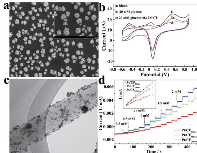
Fig. 8 (a) SEM image of Pt nanoflowers.<sup>77</sup> (b) CV curves of the Pt nanoflower electrode in 0.2 M neutral PBS.<sup>77</sup> (c) TEM image of the Pt nanoparticles on carbon fibers.<sup>80</sup> (d) Amperometric current-time response of Pt/CF in 0.1 M NaOH solution after the successive injection of different concentrations of glucose.<sup>80</sup> Reproduced ref. 77 and 80 with permission from Elsevier B.V., copyright 2011, 2015.
