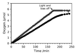
Fig. 11 Amount of  $O_2$  gas evolved at 1.23  $V_{\text{RHE}}$  under simulated sunlight (AM 1.5G, 100 mW cm $^{-2}$ ). The amount of  $O_2$  quantified with a fluorescence probe is represented by solid markers, whereas the theoretical amount of  $O_2$  calculated assuming a 100% faradaic efficiency is shown with empty markers.
