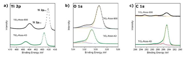
Fig. 5 XPS spectra of (a) Ti 2p, (b) O 1s and (c) C 1s of TiO<sub>2</sub>-Rose-800 and TiO<sub>2</sub>-Rose-AD. Scattered points correspond to raw data acquired in the measurements and solid lines to the fitted values.
