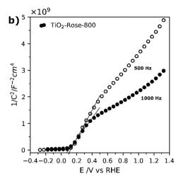
Fig. 10 (a) Nyquist plots of  $TiO_2$ -Rose-800 at the open circuit potential (OCP) of the cell under 1 sun illumination (AM 1.5G, 100 mW cm<sup>-2</sup>). (b) Mott–Schottky plots at a fixed frequency of 500 Hz and 1000 Hz of  $TiO_2$ -Rose-800 in 1 M KOH (pH = 13.6).
