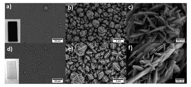
Fig. 2 SEM micrographs of  $TiO_2$  photoanodes grown by AA-CVD. (a-c)  $TiO_2$ -Rose-AD and (d-f)  $TiO_2$ -Rose-800. Insets in (a) and (d) show photographs of  $TiO_2$ -Rose-AD and  $TiO_2$ -Rose-800 photoanodes, respectively.
