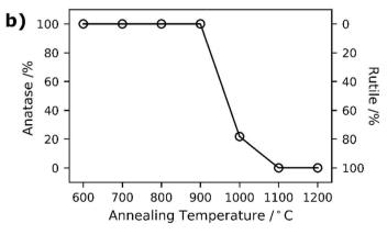
Fig. 6 (a) XRD patterns of  $TiO_2$ -Rose-800 and  $TiO_2$ -Rose-AD photoanodes prepared using  $Ti_7O_4$ (OEt)<sub>20</sub>. Standard powder pattern of anatase  $TiO_2$  is shown as well as XRD pattern of FTO-ABS. Dot: FTO-ABS diffraction peak. (b) Percentage of anatase  $TiO_2$  as a function of annealing temperature for  $TiO_2$ -Rose photoanodes.
