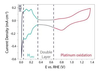
Fig. 1 Cyclic voltammogram recorded on a Pt(pc) electrode at 50 mV s<sup>-1</sup> in a 0.5 M  $H_2SO_4$  solution degassed with argon.
