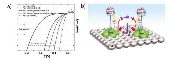
Fig. 5 (a) HER activity in alkaline solutions measured on a Pt(111) single crystal electrode, customized with different oxophilic groups and (b) "bifunctional" mechanism responsible for the enhanced activity when groups that promote water dissociation are present on the Pt(111) surface (reproduced from ref. 33 with permission from AAAS, Copyright (2011)).
