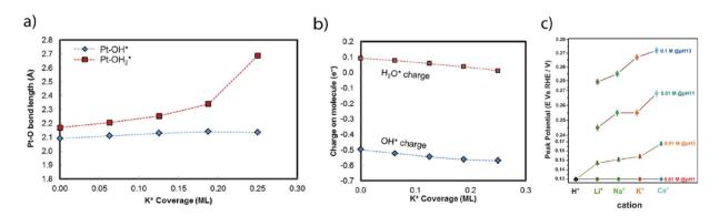
Fig. 6 (a) Pt-O bond lengths and (b) Bader charge for adsorbed OH and  $H_2O$  molecules on Pt(100) calculated using DFT at different adsorbed potassium coverages (reproduced from ref. 16 with permission from the American Chemical Society, Copyright (2016)), and (c) experimental position of the OH<sub>ad</sub>/H\* peak on Pt(533)<sub>ad</sub> at different pH values with different alkali cation contents (reproduced from ref. 17 with permission from John Wiley and Sons, Copyright (2017)).
