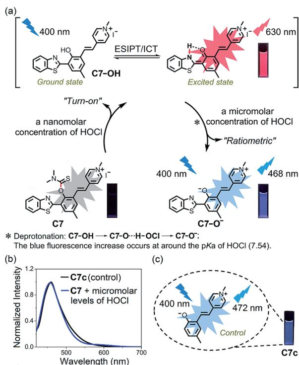
Fig. 4 (a) Proposed detection mechanism of **C7** for distinct concentration ranges of HOCl. The photographs were taken under illumination with a UV lamp (365 nm); (b) normalized fluorescence spectra of **C7c** and **C7** with addition of micromolar concentrations of HOCl (330  $\mu\text{M}$ ); (c) the photograph of **C7c** illuminated by a UV lamp (365 nm).
