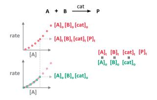
Fig. 2 The "same excess" experiments lead to the comparison of sections of the reaction profiles of reactions having the same concentration of reactants, but different concentration of product and different turnovers performed by the catalyst.
