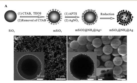
Fig. 13 (A) Schematic illustration of the procedure for the preparation of mSiO<sub>2</sub>@NH<sub>2</sub>@Ag. (B) SEM image of mSiO<sub>2</sub> microspheres. (C) SEM image of mSiO<sub>2</sub>@NH<sub>2</sub>@Ag. The insets show the low-magnification and high-magnification TEM images of mSiO<sub>2</sub>@NH<sub>2</sub>@Ag<sup>41</sup> (adapted with permission from Royal Society of Chemistry, 2015).
