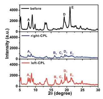
Fig. 3 XRD spectra of Azo-DF xerogels before and after 3 h irradiation of right- or left-CPL, light intensity: 5 mW cm<sup>-2</sup>.
