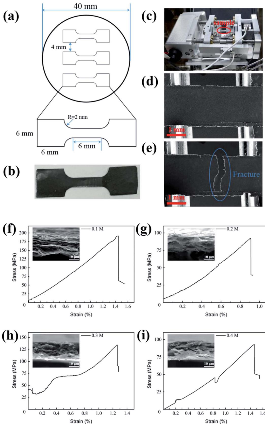
**Fig. 2** (a) The blueprint of GP sample. (b) The prepared GP strip. (c) *In situ* specimen tensile stage integrated in SEM, strip before (d) and after (e) fracture from tensile loading. (f–i) Stress–strain curves for samples at preparation condition: 0.1 mol L<sup>-1</sup> (M) K<sub>2</sub>SO<sub>4</sub>, 0.2 M, 0.3 M, 0.4 M and the SEM images (insets) of fracture surface morphology.
