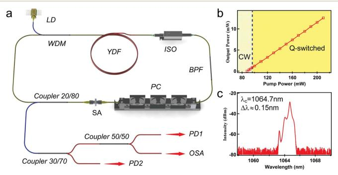
Fig. 3 (a) Experimental setup for the Yb-doped all-fiber ring laser based on BP-SA. LD: laser diode; WDM: wavelength division multiplexing; YDF: Yb-doped fiber; PI-ISO: polarization-insensitive isolator; BPF: band-pass filter; PC: polarization controller; OSA: optical spectrum analyser; and PD: photodetector. (b) Relation between output power and input power and (c) spectrum of the laser.
