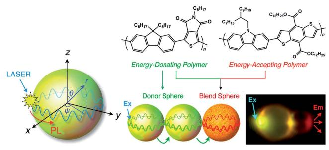
Fig. 8 Schematic diagram of a WGM inside a microsphere. PL: photoluminescence; WGM: whispering gallery mode. Adapted with permission from ref. 85. Copyright 2016 American Chemical Society.
