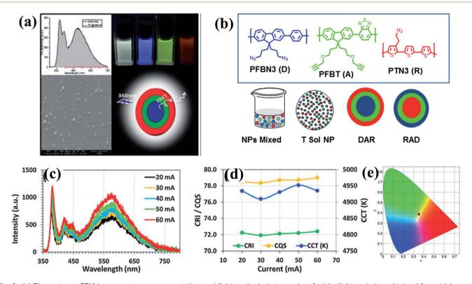
Fig. 6 (a) PL spectrum, SEM image, cartoon representation and light excited photographs of white light emission obtained from tri-layered CPNs; (b) molecular structures of conjugated polymers and four different designs to generate white light emission; (c) spectra; (d) CRI, CQS, and CCT of the tandem nanoparticle integrated white light-emitting diode at varying current levels; and (e) corresponding CIE coordinates. Adapted with permission from ref. 93. Copyright 2015 Royal Society of Chemistry.
