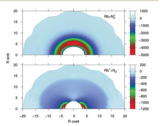
Fig. 1 Contour plots for the computed potential energy surfaces for the processes of the present study. Distances in Å and potential values in  $\rm cm^{-1}$ .
