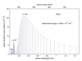
Fig. 7 Partial 'vibrational' RA cross sections corresponding to the  $R_8$  transition of collinear arrangement, as a function of the emitted photon energies and wave-lengths in the trap. The energies are given in meV (top) and the wave-lengths in mm (bottom). The initial kinetic energy of the colliding partners is also given in the figure.
