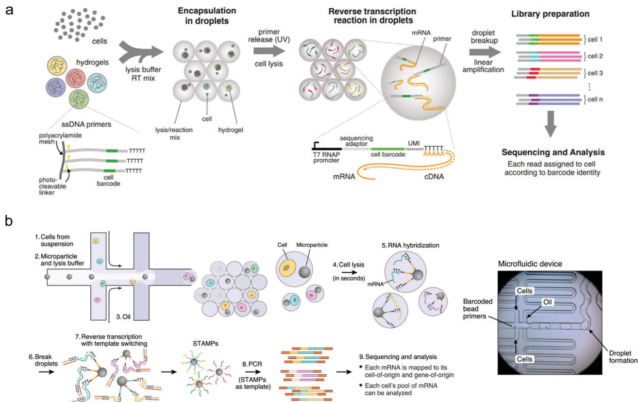
**Fig. 2** Droplet sequencing for high-throughput single-cell analysis: (a) Method based on the use of hydrogel barcodes containing DNA primers (inDrop) and (b) method based on microparticles (Drop-seq). Barcode or microparticles are delivered into droplets containing cells, lysis buffer and RT-PCR buffer, using a flow-focusing platform. Linear PCR is used for sequence analysis. Images adapted with permission from ref. 51 and 52, from Elsevier.
