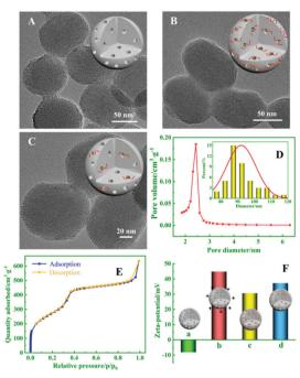
Fig. 3 TEM images of MSNs (A), CsDNA-capped PMSNs (B), and CsDNAcapped PMSNs in the presence of miRNA-21 (C); (D) pore size distribution (inset: size distribution of MSNs) and N2 adsorption-desorption isotherm of MSNs (E); and (F) zeta potentials of MSNs (a), PMSNs (b), CsDNA-capped PMSNs (c), and CsDNA capped PMSNs incubated with miRNA-21 (d).
