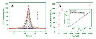
Fig. 4 (A) ECL responses of the biosensor for different concentrations of TB (pM): (a) 0, (b) 0.0005, (c) 0.001, (d) 0.01, (e) 0.1, (f) 1, (g)10, (h) 100, (i) 1000, and (j) 10000. (B) Relationship between ECL response changes (ΔECL) and the concentration of TB (0.001–1000 pM), inset: the logarithmic calibration curve for TB detection (PMT = -800).
