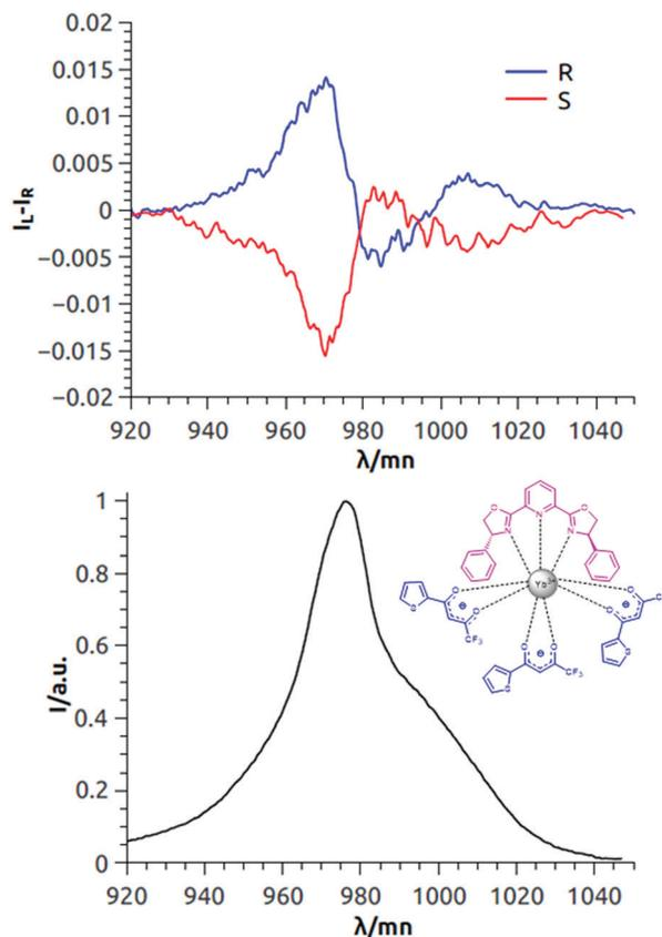
Fig. 2 Top: NIR-CPL spectra of both the enantiomers of  $\text{Yb}(\text{TTA})_3\text{PhPyBox}$ ; bottom: total NIR emission. The spectra are measured in 6 mM  $\text{CH}_2\text{Cl}_2$  solution under 365 nm irradiation (room temperature).
