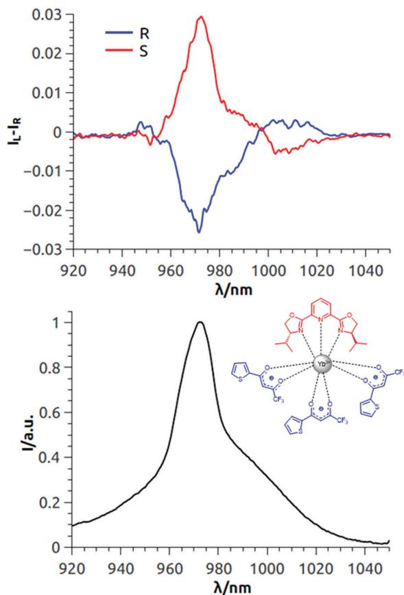
Fig. 1 Top: NIR-CPL spectra of both the enantiomers of  $\text{Yb}(\text{TTA})_3^1\text{PrPyBox}$ ; bottom: total NIR emission. The spectra are measured in 6 mM  $\text{CH}_2\text{Cl}_2$  solution under 365 nm irradiation (room temperature).
