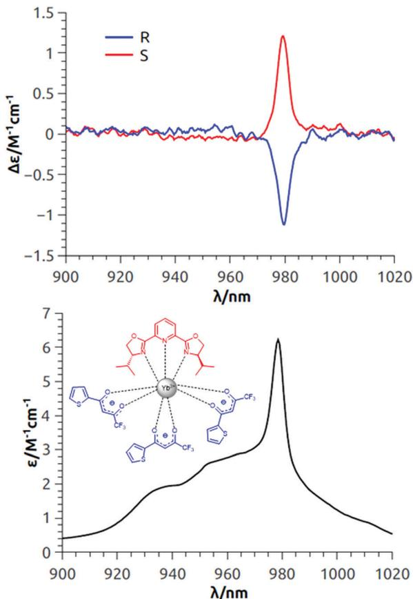
Fig. 3 Top: NIR-ECD spectra of both the enantiomers of  $\text{Yb}(\text{TTA})_3\text{PrPyBox}$ ; bottom: total NIR absorption. The spectra are measured in 7 mM  $\text{CH}_2\text{Cl}_2$  solution (room temperature).
