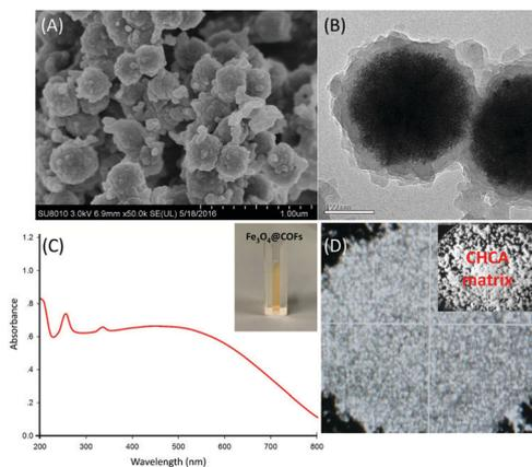
Fig. 1 (A) SEM and (B) TEM images of  $\text{Fe}_3\text{O}_4\text{@COFs}$ ; (C) UV-visible spectrum of a  $1 \text{ mg mL}^{-1}$   $\text{Fe}_3\text{O}_4\text{@COFs}$  suspension; (D) an optical image of  $1 \text{ mg mL}^{-1}$   $\text{Fe}_3\text{O}_4\text{@COFs}$ .
