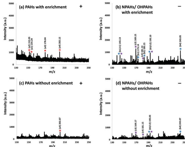
Fig. 3 Real sample SALDI-TOF-MS spectra with (a and b) and without (c and d) enrichment using  $\text{Fe}_3\text{O}_4@\text{COFs}$  ((a1) acenaphthylene; (a2) biphenyl; (a3) phenanthrene; (a4) pyrene; (b1) 1-nitronaphthalene; (b2) 3-nitrodibenzofuran; (b3) 9-nitroanthracene; (b4) 7-nitrobenz[*a*]anthracene; (c1) 2-hydroxynaphthalene; (c2) 2-hydroxyphenanthrene; (c3) 4-hydroxybiphenyl; (c4) 3-hydroxyfluorene).
