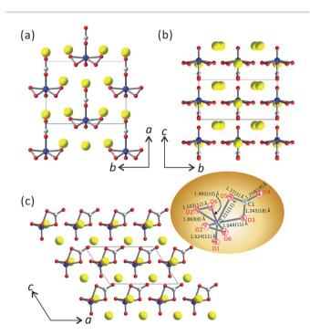
Fig. 1 Ball-and-stick models of  $Cs_3VO(O_2)_2CO_3$  in the (a) ab plane, (b) bc plane, and (c) ac plane (yellow, Cs; blue, V; gray, C; and red, O). The  $[VO(O_2)_2CO_3]$  units align parallel to  $CO_3$  groups and orient in the same direction.
