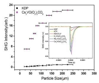
Fig. 4 Phase-matching curve for  $Cs_3VO(O_2)_2CO_3$ . The inset reveals oscilloscope traces showing the SHG intensity for  $A_3VO(O_2)_2CO_3$  (A = K, Rb, and Cs). The SHG intensities for KDP, KTP, and KSrCO<sub>3</sub>F are also plotted for comparison.
