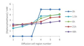
Fig. 6 Concentration profiles of diphenylmethane between regions 1 and 6 of the diffusion cell. At the start of the experiment, diphenylmethane is loaded in regions 4-6 of the cell. The points in these graphs are joined together solely as a guide to the eye.
