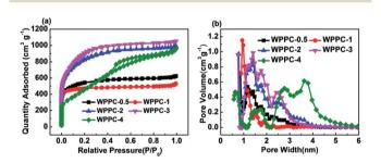
Fig. 2 (a)  $\ensuremath{N_2}$  sorption isotherms and (b) pore size distribution of the WPPCs.
