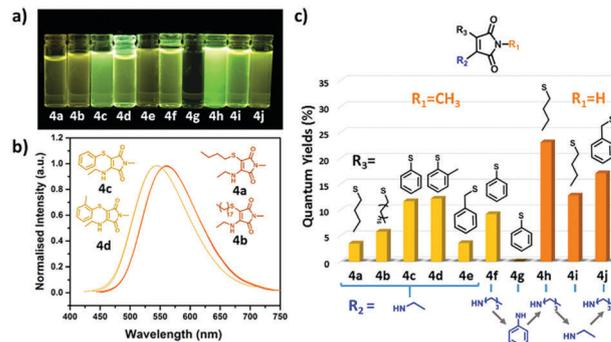
Fig. 2 (a) Solution of **ATMs** under UV light (365 nm); (b) emission spectra of different alkyl thiol (**4a–b**) and thiophenol (**4c–d**) aminomaleimides (recorded at 10  $\mu$ M in diethyl ether); (c) fluorescence quantum yields of studied **ATMs** in diethyl ether.
