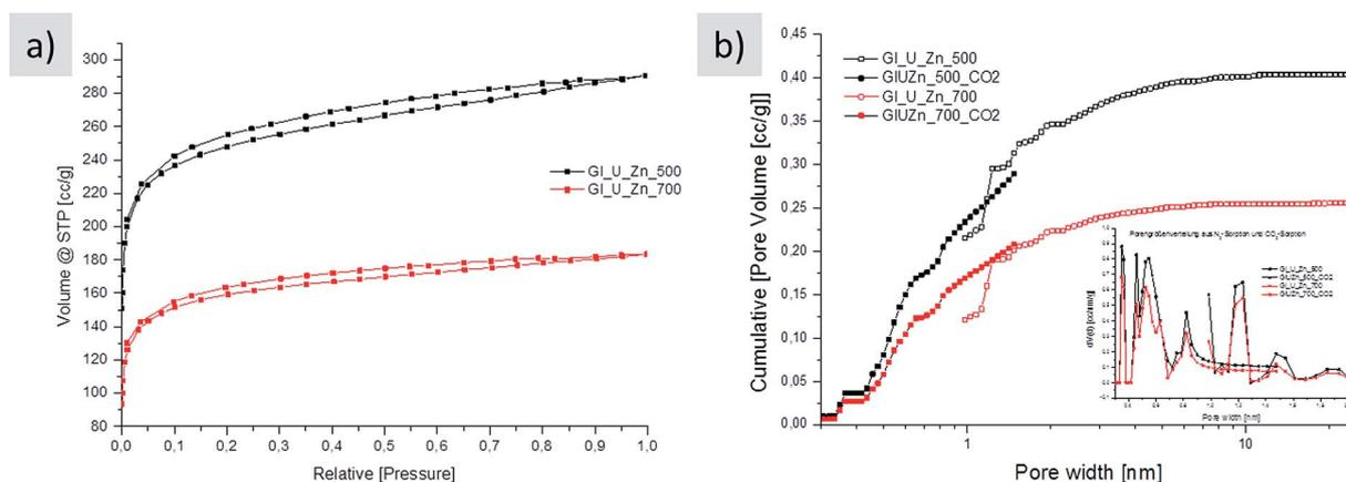
Fig. 3 (a) Nitrogen sorption isotherms and (b) pores size distribution from nitrogen (open circles) and CO<sub>2</sub> (filled circles) sorption of carbons made from glucose, urea, and ZnCl<sub>2</sub> carbonized at 500 °C (black) and 700 °C (red).
