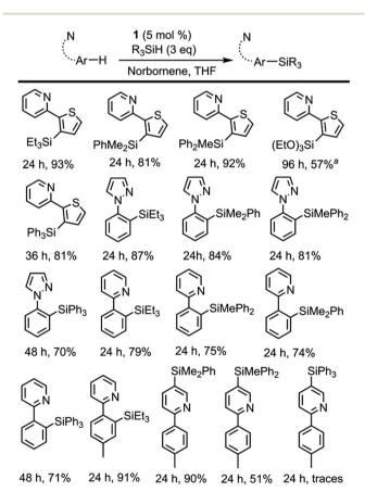
Scheme 2 Directed dehydrogenative silylation of aromatic and heteroaromatic rings. Reaction conditions: cat 1 (5 mol%), norbornene (0.40 mmol), arene (0.13 mmol), R $_3$ SiH (0.40 mmol) in THF (2 mL) at 110 °C. Isolated yields are shown. <sup>a</sup> Yield determined by  $^1$ H NMR using THF-d $_8$ .
