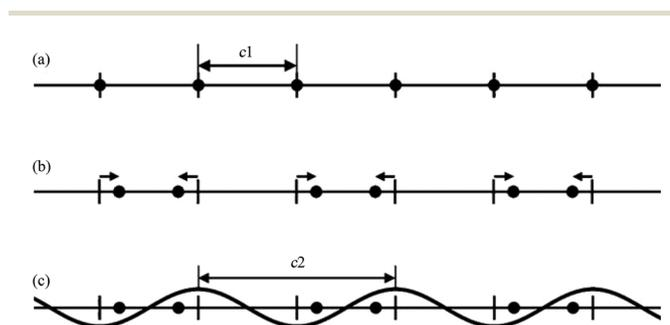
**Fig. 1** A simple 1D modulated system. (a) Before modulation: all atoms (filled circles) lie equally spaced along a straight line. (b) After modulation: half the atoms shift to the left, and half to the right (arrows). (c) Modulation in (b) represented as a simple cosine function. Reproduced with permission from ref. 16. Copyright 2007 Wiley-VCH.
