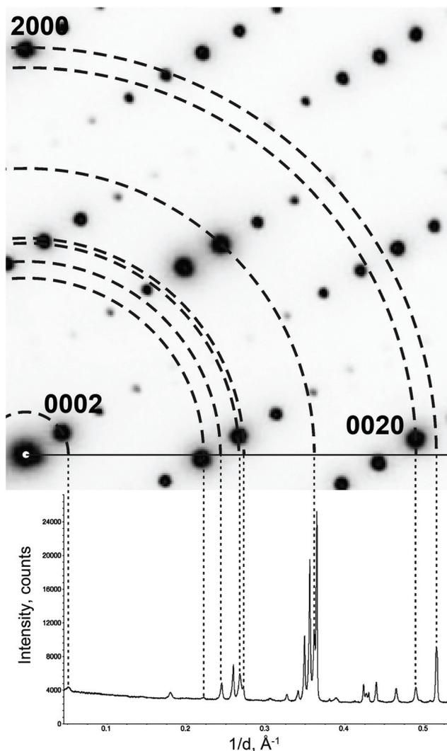
**Fig. 5** Projecting an electron diffraction pattern on a powder X-ray diffraction pattern. Note that not all reflections on the powder pattern are present on the electron diffraction pattern. These reflections belong to other reciprocal lattice sections. Reproduced with permission of the International Union of Crystallography from ref. 27.
