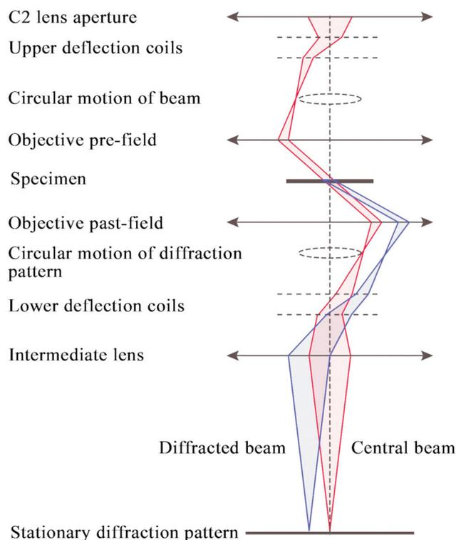
**Fig. 6** Schematic ray diagram for precession electron diffraction (PED), illustrating the rocking/de-rocking action of the beam before and after the specimen.<sup>65</sup>
