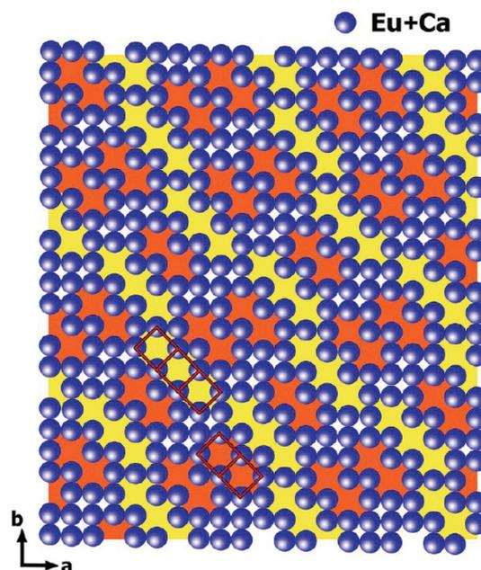
**Fig. 8** Outline of cation-vacancy ordering in the  $7a \times 9b \times 1c$  commensurate approximant.  $\text{WO}_4$  tetrahedra are not shown. The dimers (marked in orange) and trimers (marked in yellow) of the vacant cationic columns are marked with red rectangles. Reproduced with permission from ref. 66. Copyright 2013 American Chemical Society.
