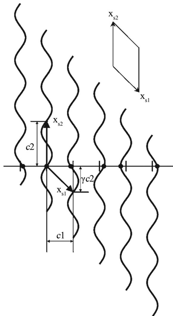
**Fig. 2** A simple 1D MS represented as a (1 + 1)D crystal. Atoms (filled circles) lie at the intersection of the horizontal line (the physical space) with a set of vertical periodic displacement functions. Drawn in this fashion, an oblique 2D unit cell with unit cell vectors  $x_{s1}$  and  $x_{s2}$  can be discerned. Reproduced with permission from ref. 16. Copyright 2007 Wiley-VCH.
