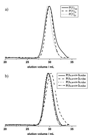
Fig. 2 SEC traces (RI detection) of (a) P(1)n and (b)  $P(1_x-co-2_y)_n$  in DMF at 333 K (the indices x and y represent the relative copolymer composition whereas n represents the degree of polymerization).
