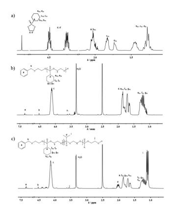
Fig. 1 (a)  ${}^{1}$ H (500 MHz) NMR spectrum of (1) in CDCl<sub>3</sub> at 298 K; (b)  ${}^{1}$ H (500 MHz) NMR spectrum of P(1) in DMSO-d6 at 298 K; (c) <sup>1</sup>H (500 MHz) NMR spectrum of P(1<sub>0.49</sub>-co-2<sub>0.51</sub>)<sub>60</sub> in DMSO-d<sub>6</sub> at 298 K.
