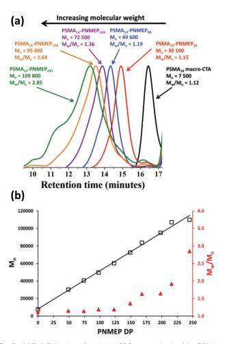
Fig. 2 (a) 3:1 Chloroform/methanol GPC curves obtained for PSMA<sub>14</sub>–PNMEP<sub>x</sub> diblock copolymer nanoparticles prepared at 10% w/w solids via RAFT dispersion polymerisation of NMEP at 90 °C. (b) Relationship between target PNMEP DP and GPC  $M_{\rm n}$  (black squares) and  $M_{\rm w}/M_{\rm n}$  (red triangles) for the same series of PSMA<sub>14</sub>–PNMEP<sub>x</sub> diblock copolymer nanoparticles prepared at 10% w/w solids.
