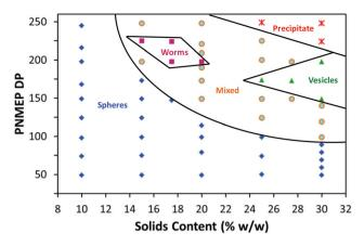
Fig. 5 Phase diagram for a series of PSMA<sub>14</sub>-PNMEP<sub>x</sub> diblock copolymers synthesised by RAFT dispersion polymerisation of NMEP in n-dodecane at various concentrations ranging between 10 and 30% w/w solids. Post-polymerisation analysis of each diblock copolymer dispersion by TEM determined the phase boundaries.
