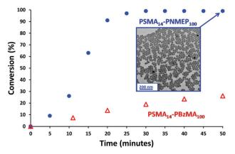
Fig. 1 Kinetics of the polymerisation of NMEP and BzMA at 90 °C when targeting PSMA $_{14}$ -PNMEP $_{100}$  (blue circles) and PSMA $_{14}$ -PBzMA $_{100}$  (red triangles) at 20% w/w solids. Insert: transmission electron microscopy image obtained after 50 min for PSMA $_{14}$ -PNMEP $_{100}$  showing the formation of near-monodisperse spherical nanoparticles with a mean diameter of 27 nm.
