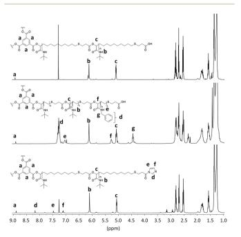
Fig. 2 <sup>1</sup>H NMR spectra of star-shaped homopolymer P10, star shaped copolymer P11 and esterified star-shaped homopolymer P12.
