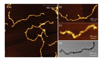
Fig. 5 AFM images of the nanostructures from PPP(EH)-b-P3MTs on HOPG: (a) PPP(EH) $_{100}$ -b-P3MT $_{90}$ , (b) PPP(EH) $_{100}$ -b-P3MT $_{130}$ . (c) High-resolution AFM images of the nanostructures from PPP(EH) $_{100}$ -b-P3MT $_{130}$ . (d) TEM images of the nanostructures from PPP(EH) $_{100}$ -b-P3MT $_{130}$  on a Cu/C TEM grid.
