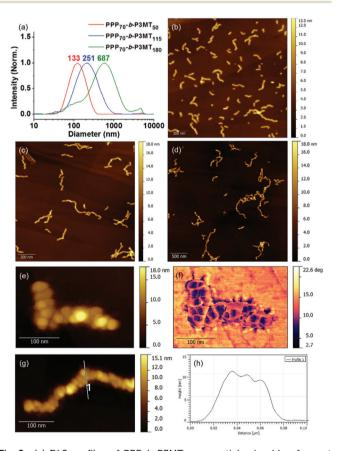
Fig. 2 (a) DLS profiles of PPP-b-P3MT nanoparticles in chloroform at 20 °C. AFM images of the nanostructures from PPP-b-P3MTs on HOPG: (b)  $PPP_{70}-b-P3MT_{50}$ , (c)  $PPP_{70}-b-P3MT_{115}$  and (d)  $PPP_{70}-b-P3MT_{180}$ . High-resolution AFM (e) height and (f) phase images of the nanostructures from PPP<sub>70</sub>-b-P3MT<sub>115</sub>. (g) High-resolution AFM image and (h) height profile of the nanostructure from PPP<sub>70</sub>-b-P3MT<sub>115</sub>.
