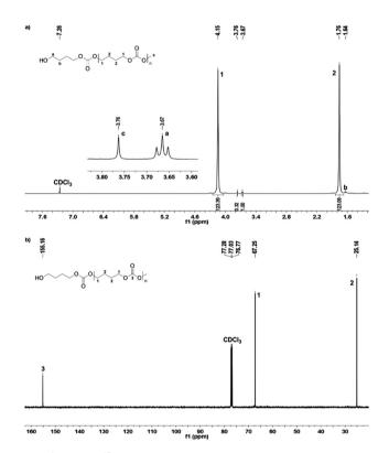
Fig. 2 <sup>1</sup>H (a) and <sup>13</sup>C NMR (b) spectra of PBC 9
