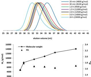
Fig. 3 SEC traces and plot  $M_n$  (determined by SEC) and the dispersity values of PBC 9 versus the polymerization time in the 2nd step.
