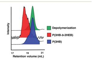
Fig. 2 GPC traces of P(3HB) and P(2HEB) copolymers and depolymerisation.
