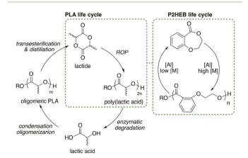
Scheme 2 Idealized life cycles of poly(lactic acid) and poly(2-(2-hydroxyethoxy)benzoate) moving from four energy intensive steps in PLA recycling to simple ring-opening polymerization and ring closing depolymerization steps for P2HEB.
