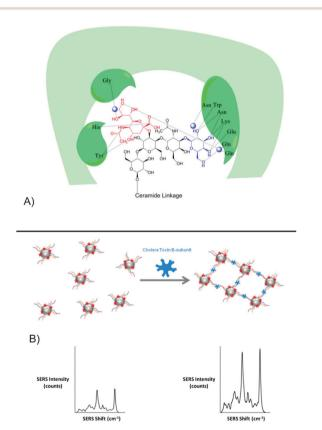
Fig. 1 (A) GM1-CTB binding pocket structure (H-bonding) with sialic acid (red) and galactose (blue) residues shown. Water is shown as blue spheres. (B) Galactose and sialic acid linkers (orange and purple chains respectively) are used to coat the nanoparticles prior to incubation with CTB. The close proximity of the nanoparticles following aggregation with CTB results in "hot-spots" of electromagnetic energy which increase the scattering intensity of surface bound RB1 (red stars) SERS signal.
