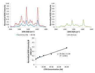
Fig. 3 RB1 SERS spectra of GSNPs before and after addition of (top left) CTB or (top right) ConA in synthetic freshwater. (Lower middle) Normalised SERS Intensity of 1364 cm<sup>-1</sup> peak measured 5 minutes after addition of the indicated concentration of CTB with 5 replicates per concentration. The limit of detection determined is 1 nM. The laser excitation wavelength used is 514.5 nm with a 1 second acquisition and 3 accumulations, 5 replicates measured
