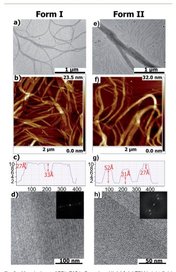
Fig. 2 Morphology of PBI-C10 in Form I and II. (a)  $\theta$  (e) TEM bright field images; (b)  $\theta$  (f) AFM images; (c)  $\theta$  (g) section profile of an AFM topographic image showing the presence of characteristic terraces; (d), (h) low dose HR-TEM images (inset: fast Fourier transform). In Form II, note the presence of some intense reflections in the first layer line above the equator which is a fingerprint of a helical molecular packing.
