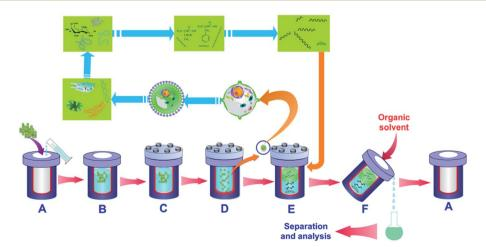
Fig. 10 Experimental procedure of HTL for microalgae in closed batch reactor (A) reactor, (B) charging, (C) sealing, (D) heating, (E) cooling, (F) washing.
