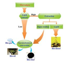
Fig. 4 Possible microalgal processing options based on lipid content.
