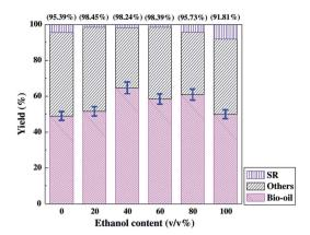
Fig. 12 Effect of ethanol content on the bio-oil, others and SR yields for the microalgae liquefaction in ethanol-water cosolvent.<sup>175</sup> Copyright 2012 Elsevier.
