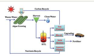
**Fig. 11** Concept of Environment-Enhancing-Energy (E<sup>2</sup>-Energy) technology.<sup>42</sup> Copyright 2011 Royal Society of Chemistry.
