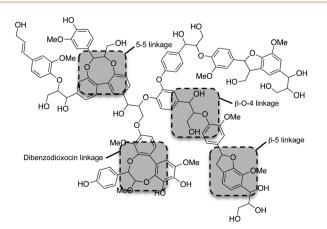
Fig. 4 Schematic representation of lignin chemical bonds.
