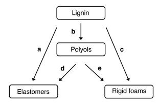
**Fig. 6** Synthetic routes for lignin incorporation in polyurethane materials: (a) direct use, (b) synthesis of liquid polyol, (c) synthesis of rigid polyurethane foams using lignin-based polyols, (e) synthesis of polyurethane elastomers using lignin-based polyols and (d) synthesis of rigid polyurethane foams using lignin as reactive filler.<sup>98</sup>
