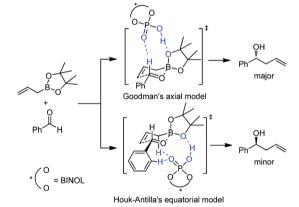
Scheme 23 Transition state of chiral BINOL-phosphoric acid catalyzed allylboration.
