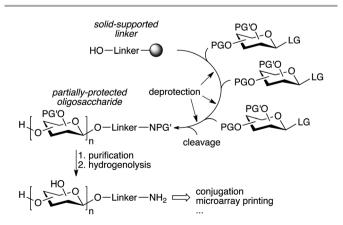
Fig. 4 Streamlined automated solid-phase oligosaccharide synthesis (PG': protecting group labile to hydrogenolysis).69
