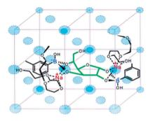
Fig. 9 Glucose binding to two boronic acid moieties of BA-PEG-AA. The binding motif is stabilised by PEG-Na+ complex. Reproduced with permission from Anal. Chem., 2003, 75, 2316–2323. Copyright 2003 American Chemical Society.
