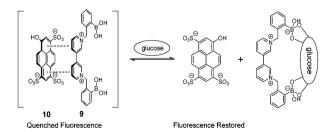
Scheme 3 Glucose-binding induced dissociation of the electrostatic assembly of 9 and 10
