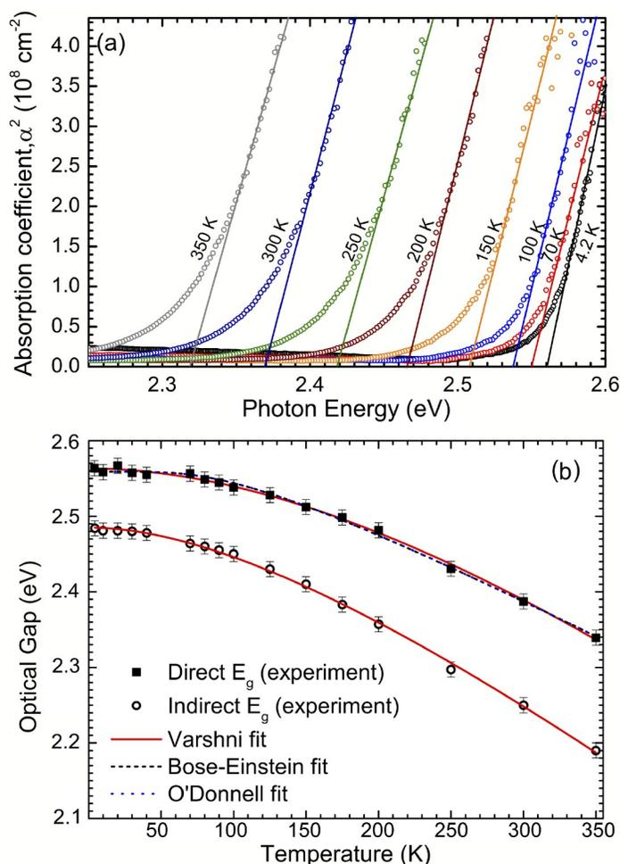
**Fig. 5** (a) Optical absorption spectra as a function of temperature and (b) corresponding direct (closed squares) and indirect (open circles) band gaps for the same single crystal of tin disulfide. Also shown are Varshni, Bose-Einstein and O'Donnell fits to the direct band gaps and a Varshni fit to the indirect band gap.
