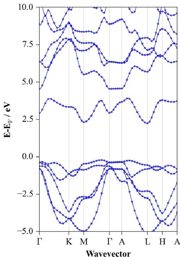
**Fig. 6** Band structure diagram of SnS<sub>2</sub> for the experimentally determined lattice constants at the HSE06/DFT level of electronic structure theory.
