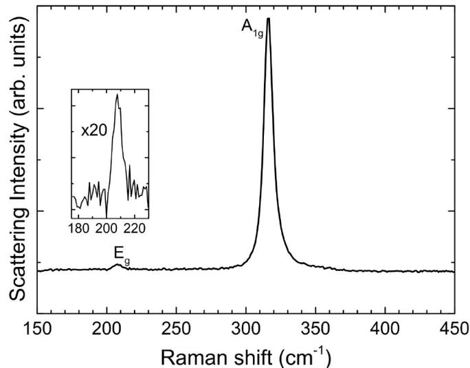
**Fig. 3** Raman spectrum from SnS<sub>2</sub>, with A<sub>1g</sub> and E<sub>g</sub> modes indicative of the 2H polytype. The inset shows a 20 times magnification of the E<sub>g</sub> mode.
