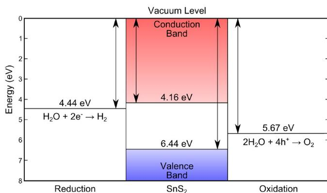
**Fig. 4** The energy levels of SnS<sub>2</sub> as determined by XPS/IPES in this work, showing the desirable band placements for water splitting.<sup>7,8</sup>
