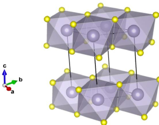
**Fig. 1** Ground state (2H) structure of SnS<sub>2</sub> showing the 2-dimensional bonded plane of edge-sharing bonded octahedra and the conventional unit cell.
