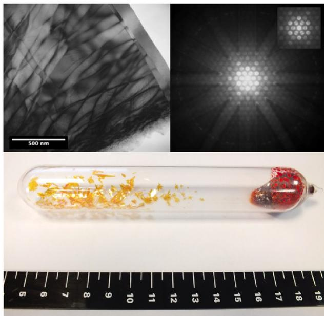
**Fig. 2** Top left - Bright field transmission electron microscopy of an SnS<sub>2</sub> platelet, image near the [0001] zone axis. Top right - Selected area diffraction pattern near the [0001] zone axis and, inset, the convergent beam electron diffraction for the same sample. Bottom centre - Macroscopic single crystals synthesised from the CVT method, with the scale in centimetres.
