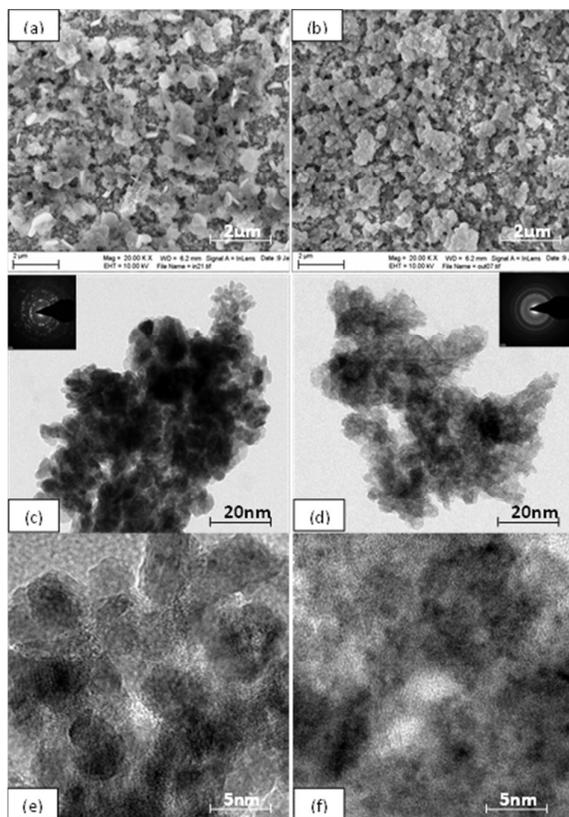
**Fig. 6:** Microscopy characterization of ZnO:Co morphologies after EPD using ethanol as electrolyte. (a) and (b) SEM surface view before and after electrochemistry, respectively. (c) and (d) corresponding TEM images of ZnO:Co lamellae before and after electrochemistry, respectively. (e) and (f) Magnified TEM images of ZnO:Co lamellae before and after the electrochemistry, respectively.
