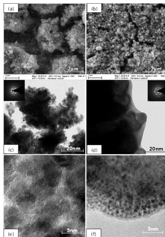
**Fig. 5:** Microscopy characterization of ZnO:Co morphologies after EPD using acetonitrile as electrolyte. (a) and (b) SEM surface view before and after electrochemistry, respectively. (c) and (d) corresponding TEM images of ZnO:Co lamellae before and after electrochemistry, respectively. (e) and (f) Magnified TEM images of ZnO:Co lamellae before and after the electrochemistry, respectively.
