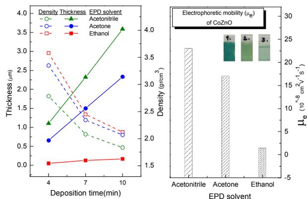
Fig. 1: (a) effect of the organic solvent and the deposition time on the thickness and the density of the layers. (b) Influence of the organic solvent on the electrophoretic mobility of ZnO:Co particles in the suspension.
