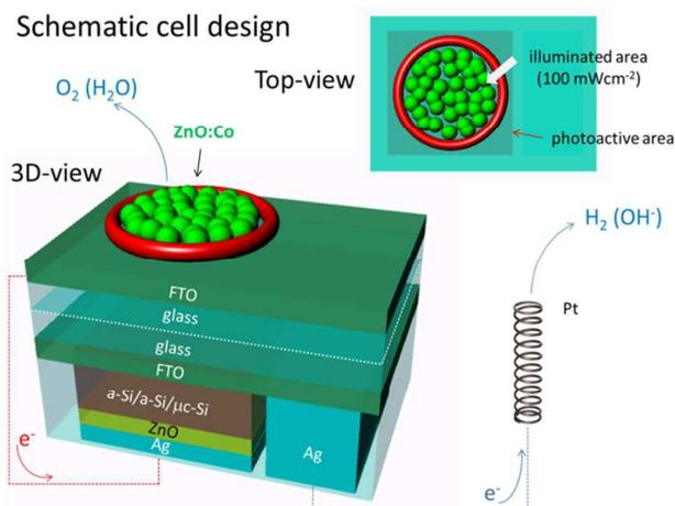
**Fig. 8:** Schematic setup of the combined junctions, an amorphous/microcrystalline silicon solar cell (bottom) and a ZnO:Co/FTO heterojunction (top). The white dashed line in the 3D-schematic indicates where the top ZnO:Co/FTO electrode can be lifted off. In the top-view, the O-ring is depicted in decreased size in order to stress the photoactive area beneath.
