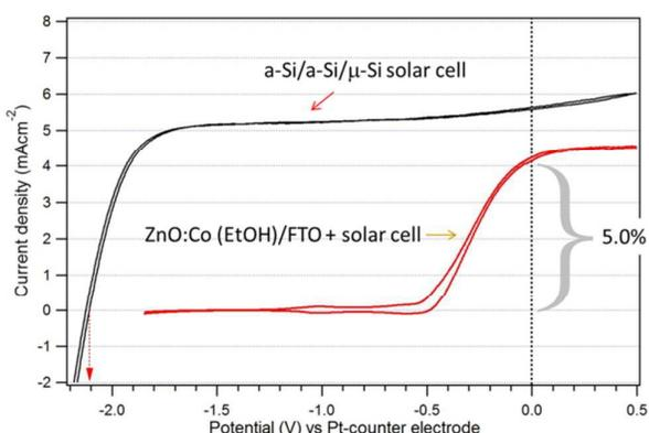
**Fig. 9:** Photocurrent-voltage behavior of ZnO:Co/FTO prepared from ethanol suspensions. The electrocatalytic layer was fixed to the photoactive front-side of the triple-junction silicon solar cell (compare Fig. 8). Short-circuit photocurrent densities of about  $4.2 \text{ mAcm}^{-2}$  result in an efficiency of 5% for direct photo-assisted water splitting.
