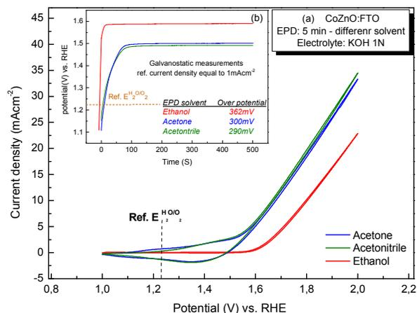
**Fig. 4:** (a) Current voltage behavior of ZnO:Co prepared in different organic solvents ethanol (red line), acetone (blue line) and acetonitrile (green line) deposited on FTO substrate. (b) Galvanostatic measurements of the layers correspond to current density of 1 mAcm<sup>-2</sup>. Electrolyte: KOH 1N.
