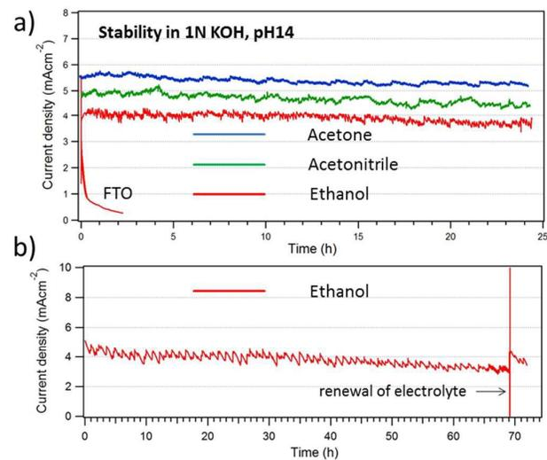
**Figure 7:** Stability assessment of ZnO:Co, prepared from ethanol-containing suspensions, at pH14. For comparison, the rapid degradation of a bare FTO substrate is indicated.
