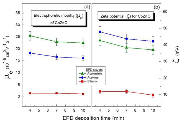
Fig. 2: (a), (b) Effect of the organic solvent as a function of deposition time on the electrophoretic mobility and the zeta potential of the ZnO:Co particles respectively.
