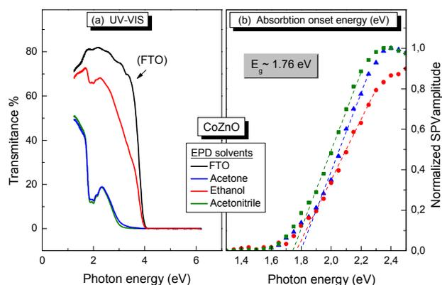
**Fig. 3:** optical characterization of ZnO:Co deposited on FTO substrate (a) Transmission spectra as a function of wavelength (b) Normalized SPV amplitudes as a function of photon energy for Ethanol (red dots), Acetone (blue dots) and Acetonitrile (green dots).
