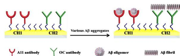
Fig.1 Schematic representation of simultaneous SPR detection of A $\beta$ (1–42) oligomers and fibrils. Carboxymethylated (CM)-dextran-covered SPR chips were modified with A11 antibody (channel 1, CH1) and OC antibody (channel 2, CH2),
