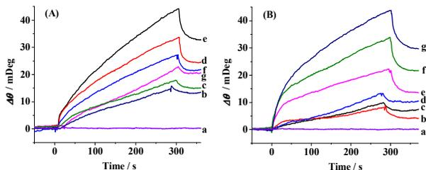
**Fig.2** SPR sensorgrams showing the capture of (A) oligomers of A $\beta$ (1–42) by A11 antibody-covered SPR chip (CH1) and (B) fibrils of A $\beta$ (1–42) by OC antibody-covered SPR chip (CH2). 10  $\mu$ M of A $\beta$ (1–42) was incubated in 10 mM phosphate buffer (pH 7.4) at 37  $^{\circ}$ C for 0 h (a), 1 h (b), 2 h (c), 4 h (d), 6 h (e), 10 h (f) and 24 h (g).
