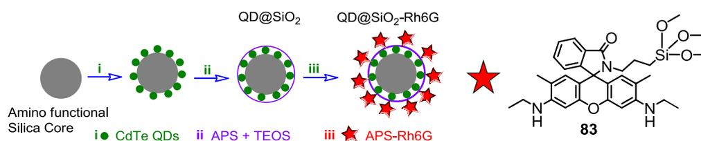
**Figure 44.** Rhodamine 6G (**83**) grafted on the silica surface in the hybrid receptor for the recognition of  $\text{Hg}^{2+}$ . Schematic representation for the methodology adopted developing  $\text{QDs@SiO}_2\text{-Rh6G}$ .
