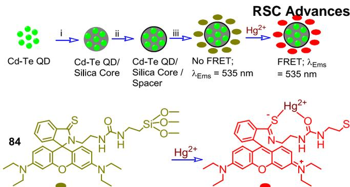
**Figure 45.** Strategy used for FRET base  $\text{Hg}^{2+}$  sensor on QDs.
