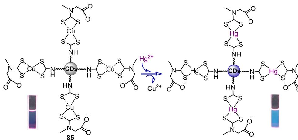
**Figure 46.** Schematic representation of ‘turn on’ response of Carbon nanodots **85** by displacement of  $\text{Cu}^{2+}$  ions by  $\text{Hg}^{2+}$  ions. Reprinted with permission from ref 76. Copyright 2014 American Chemical Society.
