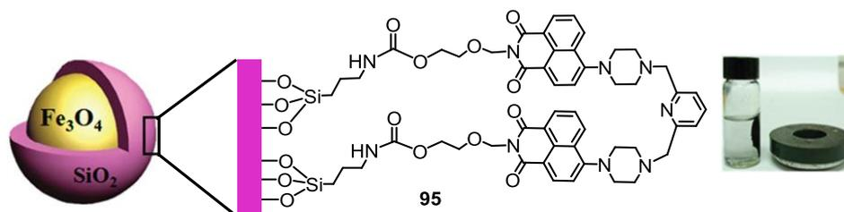
**Figure 53.** Structure of the functionalised nano particle for the detection of  $\text{Hg}^{2+}$  [Inset: Photograph of a magnet attracting **95** in water]. Reprinted with permission from ref 83. Copyright 2010 Royal Society of Chemistry.
