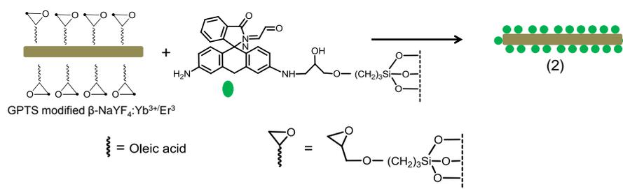
**Figure 62.** The pictorial representation of the  $\text{Hg(II)}$  sensing nanocomposite system (**103**) constructed with  $\beta\text{-GPTS}$  modified  $\text{NaYF}_4\text{:Yb}^{3+}/\text{Er}^{3+}$  nanorods and rohadimine derivative.
