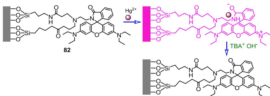
**Figure 43.** Rhodamine derivative immobilised on mesoporous silica surface, for the reversible recognition of  $\text{Hg}^{2+}$ .
