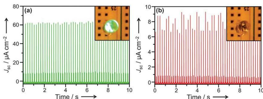
**Figure 86:** Rectified  $J_{sc}$  of the as-developed TENG before (a) and after (b) the interaction with  $5 \mu\text{M}$   $\text{Hg}^{2+}$  ions. Insets: photograph of the indicated LED lamp before (a) and after (b) interaction with  $5 \mu\text{M}$   $\text{Hg}^{2+}$  ions, as an indication of detected concentration. Reprinted with permission from ref 129. Copyright 2013 Wiley.
