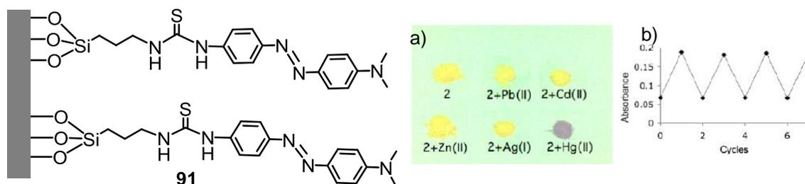
**Figure 49.** Modified mesoporous silica for chromogenic recognition of  $\text{Hg}^{2+}$ . [Inset: a) change in colour of **91** in presence of different metal ions, b) Cycles of  $\text{Hg}^{2+}$  absorption after washing with water]. Reprinted with permission from ref 79. Copyright 2013 Royal Society of Chemistry.
