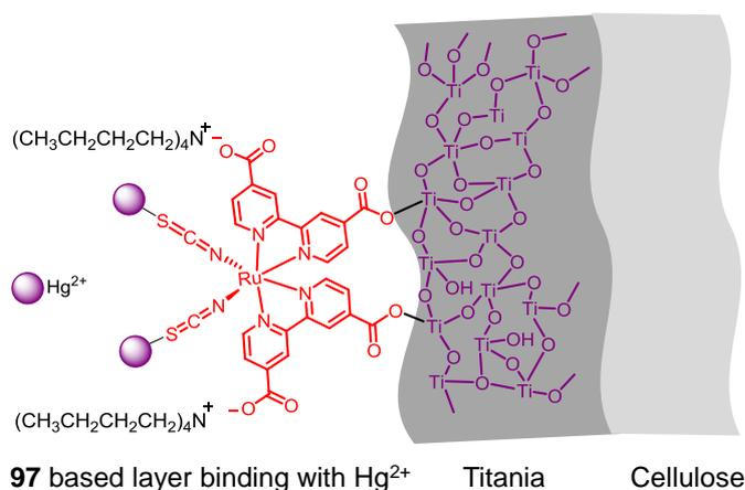
**Figure 57.**  $\text{Hg}^{2+}$  ion recognition using  $\text{TiO}_2$ -**97** multilayer modified natural cellulose substance.<sup>85</sup>
