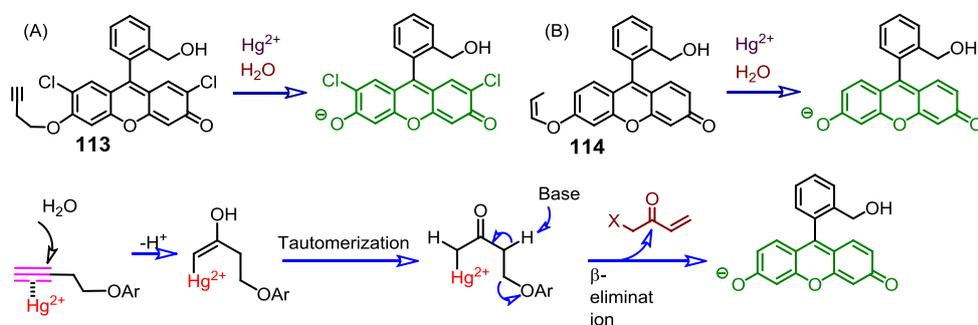
**Figure 69.** Detection of  $\text{Hg}^{2+}$  based on the of oxymercuration and demercuration reaction of electron rich  $\pi$ -bonds and the proposed mechanistic pathway for the elimination reaction.
