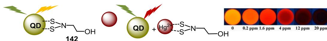
**Figure 85.** Quantum dot based  $\text{Hg}^{2+}$  sensors [Inset: colour change observed on cellulose acetate paper on dropping solution of  $\text{Hg}^{2+}$ ]. Reprinted with permission from ref 127. Copyright 2012 American Chemical Society.
