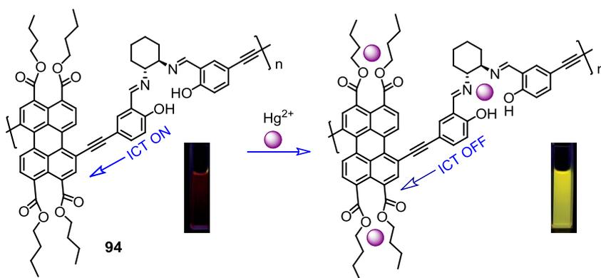
**Figure 52.** Polymer based system for the recognition of  $\text{Hg}^{2+}$  through coordination induced ICT 'ON-OFF' process. Reprinted with permission from ref 82. Copyright 2012 Royal Society of Chemistry.
