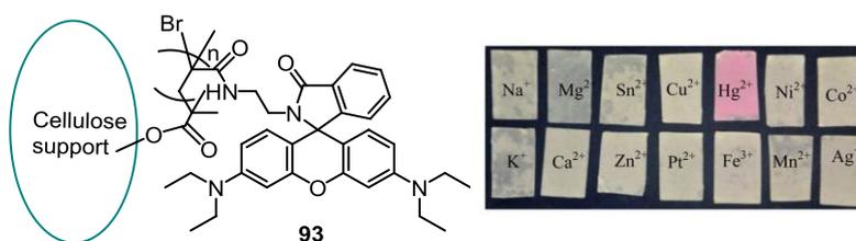
**Figure 51.** Rhodamine derivative on modified cellulose filter paper [Inset: Optical photograph of cellulose paper in presence of different metal ions]. Reprinted with permission from ref 81. Copyright 2013 Royal Society of Chemistry.
