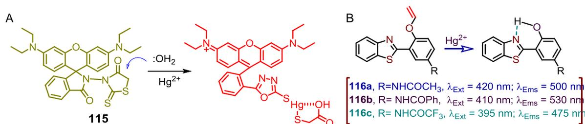
**Figure 70.** (A)  $\text{Hg}^{2+}$  mediated oxazole formation. (B)  $\text{Hg}^{2+}$  ions promoted hydrolysis of vinylic ethers and excited state intramolecular proton transfer leading to change in emission signals.
