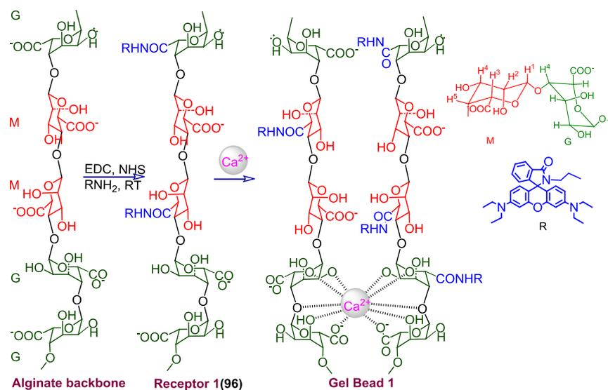
**Figure 54.** Bio-polymeric gel bead of rhodamine-alginate conjugate was used for the detection and for the removal of  $\text{Hg}^{2+}$  from its aqueous solution.<sup>84</sup>
