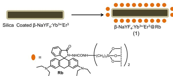
**Figure 61.** The pictorial representation of the  $\text{Hg(II)}$  sensing nanocomposite material (**102**) constructed with silica coated  $\beta\text{-NaYF}_4\text{:Yb}^{3+}/\text{Er}^{3+}$  nanorods and rohadimine derivative.
