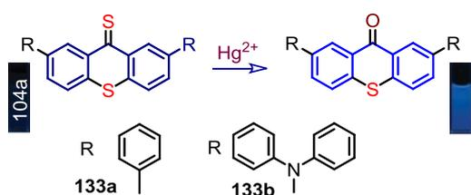
**Figure 79.** Fluorescence changes in the presence of  $\text{Hg}^{2+}$  and proposed sensing mechanism: desulfurization of **133a** and **133b**, promoted by  $\text{Hg}^{2+}$  ions. Reprinted with permission from ref 120. Copyright 2012 Royal Society of Chemistry.
