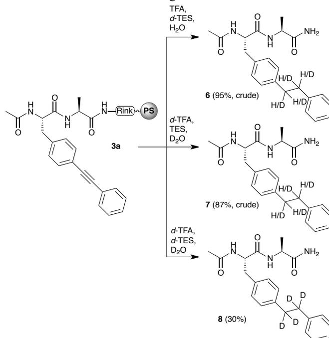
Scheme 2. Reduction of the triple bond of a resin-bound bisarylethyne-containing peptide (**3a**) by means partially deuterated mixtures of TFA/TES/water – 80/10/10 (v/v/v).
