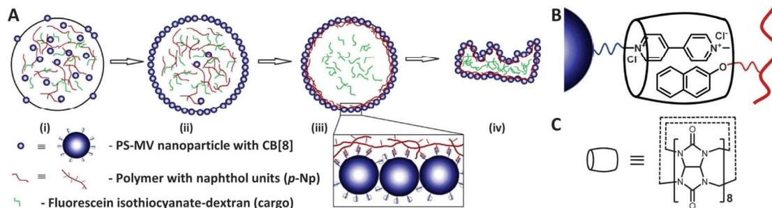
**Fig. 12** (A) Schematic of colloidosome formation; (B) ternary supramolecular complex formation between PS-MV, p-Np and CB8. (C) The molecular structure of CB8. (Reprinted with permission from ref. 63. Copyright 2014 Royal Society of Chemistry.)
