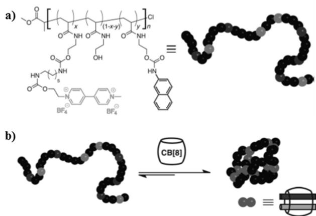
**Fig. 10 (a)** The structure of poly(N-hydroxyethyl acrylamide) polymer conjugated with guest moieties ( $MV^{2+}$  and Np) for complexation with CB8; **(b)** Single chain polymer nanoparticle formation through ternary complex of CB8. (Reprinted with permission from ref. 56. Copyright 2012 Wiley-VCH Verlag GmbH & Co. KGaA.)
