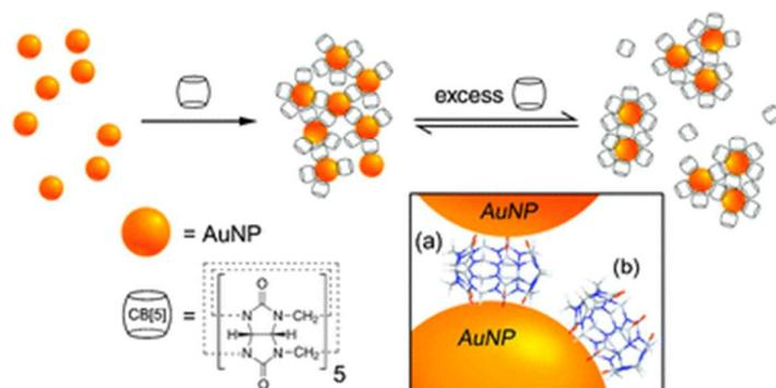
**Fig. 1** The preparation of CB5-capped gold nanoparticles and the formation of dynamic aggregates consisting of a controllable ratio of singly and doubly capped CB5. (Reprinted with permission from ref. 27. Copyright 2010 Royal Society of Chemistry.)
