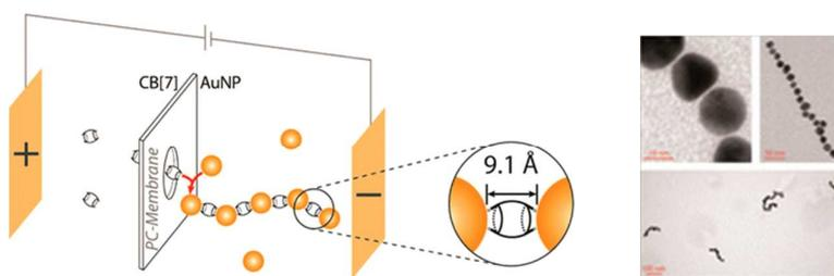
**Fig. 3** The use of CB7 as nanojunctions of 0.9 nm in the electrokinetic assembly of one-dimensional nanoparticle chains. (Reprinted with permission from ref. 38. Copyright 2013 American Chemical Society.)
