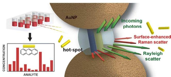
**Fig. 2** Schematic of host-guest SERS analysis using ternary complexation: CB8 aggregates AuNPs and localizes the analyte in the hot-spot for SERS analysis. (Reprinted with permission from ref. 36. Copyright 2012 American Chemical Society.)
