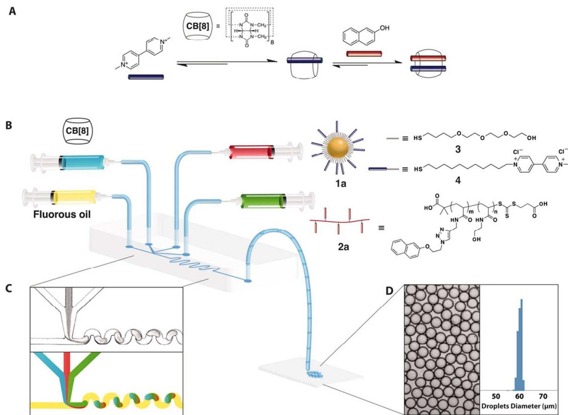
**Fig. 5** The fabrication of mono disperse supramolecular microcapsules using microfluidic approach. (A) Schematic representation of a ternary complex formation between methyl viologen dication (MV<sup>2+</sup>), 2-naphthol and CB8. (B, C, D) Microfluidic set-up for the preparation of hybrid-capsules. (Reprinted with permission from ref. 40. Copyright 2012 Science.)
