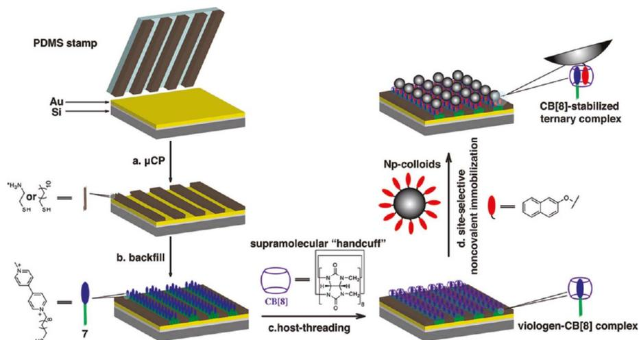
**Fig. 13** Schematic representation of site-selective noncovalent immobilization of Np-colloids on a micropatterned viologen terminated Au substrate in the presence of CB8. (Reprinted with permission from ref. 64. Copyright 2010 American Chemical Society.)
