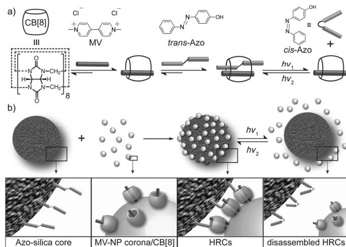
**Fig. 6** (a) Ternary complex formation between MV, trans-azo and CB8 and the disassembly of ternary complex by a light stimulus; (b) Photoresponsive hybrid raspberry-like colloids (HRCs) prepared by the host-guest chemistry of CB8. (Reprinted with permission from ref. 41. Copyright 2014 Wiley-VCH Verlag GmbH & Co. KGaA.)
