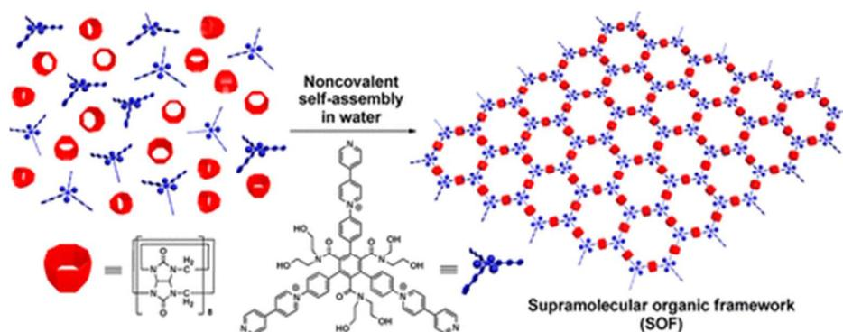
**Fig. 14** Schematic representation of CB8-mediated single-layer two-dimensional honeycomb supramolecular organic framework (SOF) formation in water. (Reprinted with permission from ref. 66. Copyright 2013 American Chemical Society.)
