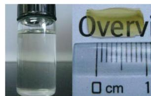
**Fig. 12**  $\text{Ce}^{3+}$ -doped nanowires in cyclohexane (left) and a film formed from  $\text{Ce}^{3+}$ -doped nanowires (right). Adapted with permission from ref. 63, Copyright 2012, Wiley Online Library.
