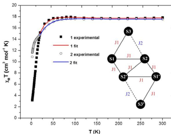
**Figure 3.** Plot of  $\chi_M T$  vs.  $T$  for complexes **1** and **2** in an applied field of 0.1 T. The inset shows the coupling scheme used to fit the data to Hamiltonian (1). See text for details.
