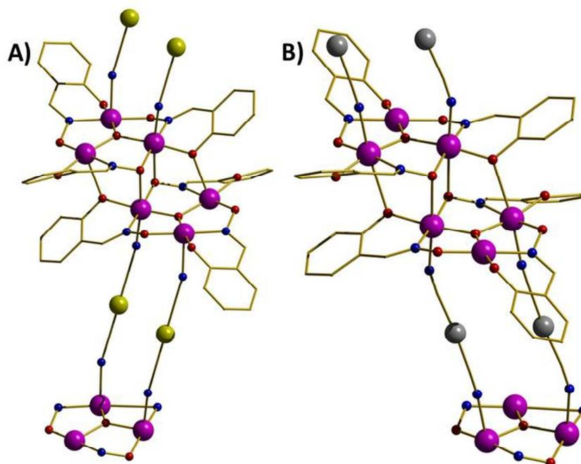
The linear  $[\text{M}(\text{CN})_2]^-$  ( $\text{M} = \text{Au}, \text{Ag}$ ) anions can be used as metalloligands in oxime-based Mn chemistry to afford 1D chains of  $[\text{Mn}^{\text{III}}_6]$  Single-Molecule Magnets (SMMs).
