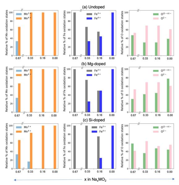
Fig. 2 Redox-active ions in (a) undoped  $Na_xFe_{0.5}Mn_{0.5}O_2$ , (b) Mg-doped  $Na_xMg_{0.11}Fe_{0.22}Mn_{0.67}O_2$ , and (c) Si-doped  $Na_xSi_{0.11}Fe_{0.22}Mn_{0.67}O_2$  showing the relative % amount of the different oxidation states of Mn, Fe and O as a function of Na content (x) from the pristine material to high charge states (x = 0.33, 0.16, 0.00).
