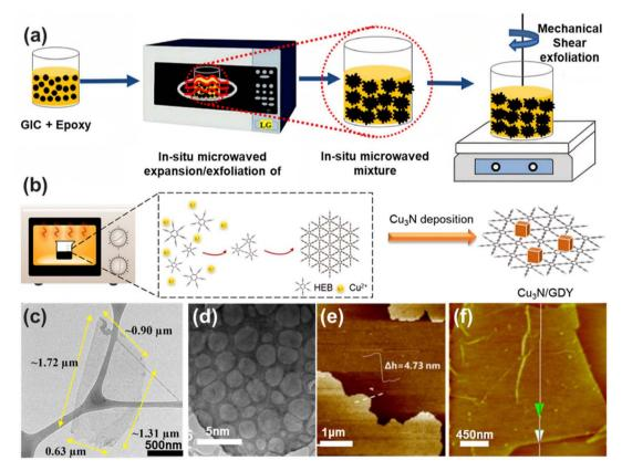
Fig. 5 (a) Schematic for preparation of epoxy/graphene nanocomposites, (b) schematic illustration of the synthesis of Cu<sub>3</sub>N/GDY, (c) TEM images of graphene platelets, (d) TEM and (e) AFM images of GDY, and (f) typical AFM height images of MW-rGO. Reproduced with permission from ref. 160. Copyright, 2024, RSC.
