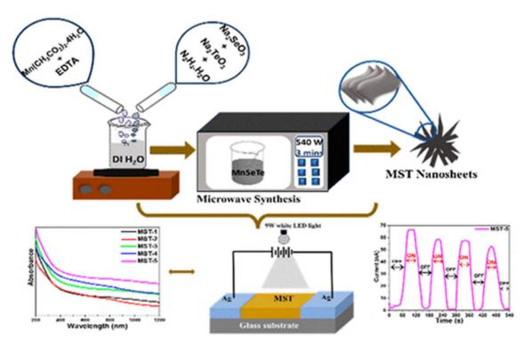
Fig. 8 Schematic representation of MAS of MnSeTe nanocomposite flowers for optoelectronic and photoresponse applications. Reproduced with permission from ref. 249. Copyright, 2024, ACS.
