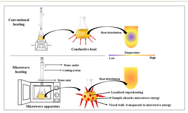
Fig. 1 Schematic representation of the mechanism of conventional and microwave heating
